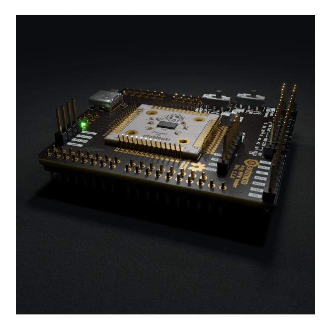
The Arty MPW tester is simple expansion board compatible with Digilent Arty A7 development kit. This board connects IO signals from the Xilinx Artix FPGA located on the Arty board to an open hardware Caravel breakout board. The Caravel breakout board allows testing ASIC designs prepared for Multi Project Wafer (MPW) shuttles and fabricated with one of the available
