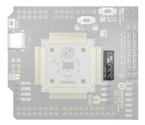
When XCLK SEL is set to INT user can enable and disable onboard oscillator using INT XCLK EN header:
